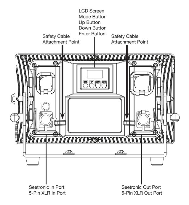
**DMX-512:** DMX is short for Digital Multiplex. This is a universal protocol used as a form of communication between intelligent fixtures and controllers. A DMX controller sends DMX data instructions from the controller to the fixture. DMX data is sent as serial data that travels from fixture to fixture via the DATA "IN" and DATA "OUT" XLR terminals located on all DMX fixtures (most controllers only have a DATA "OUT" terminal).
